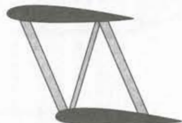
Basic N-strut Members should be well-streamlined. Used on many full-scale bipes.
