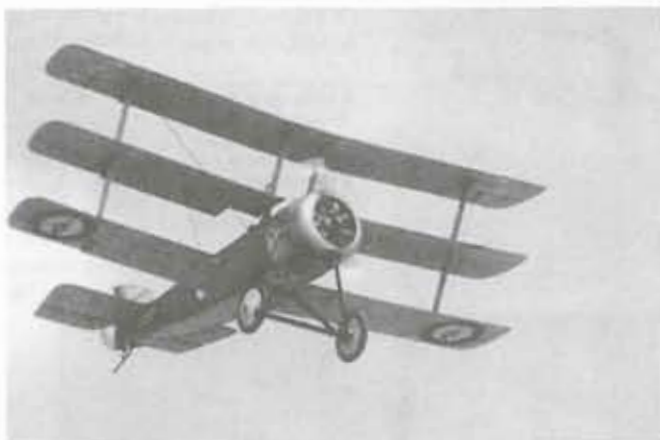
Peter McDermott's 78-inch-span, 1/4-scale Sopwith triplane took first at the '92 FAI Scale Internats in Muncie, IN. It's powered by a Laser 180 twin that spins an 18x6 Dynathrust prop.
