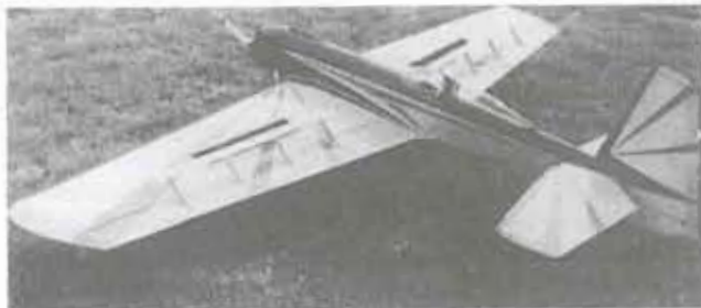
This is the author's attempt to build a monoplane that performs like a bipe: 86-inch span; 1,230-square-inch wing; 8 pounds; all-moving vertical tail; spoilers; balloon-tire retracts; and paddle balancers on ailerons. The plane is currently powered by a piped Webra 120.
