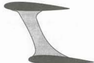
Unlited streamlined strut Used on numerous, present-day, full-scale, aerobatic bipes. May be made of 1/4-inch sheet balsa for models with .60 to 1.20 engines. Low drag and additional lateral area improve knife-edge and handling.
