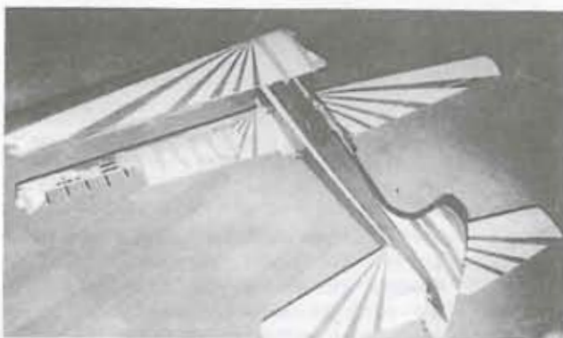
The wing flutter damage shown here occurred while the plane was flying straight and level at about 105mph. The flutter was second harmonic, caused by excess tip balance weight on long, flexible ailerons. The flutter was cured by adding mass dampers at the 40-percent-span position. The model landed safely with just one functional aileron. All damage occurred within 0.1 second. The additional wing on the bipe saved the model; this is one advantage of a biplane over a monoplane! On another occasion, the same bipe landed safely after losing the entire upper wing, part of the lower wing and half the stab in a midair collision!
