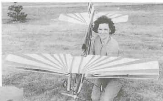
A 68-inch-span biplane designed by the author for .60 to .73 2-stroke power, shown here with a Weber .73 and quiet muffler. Doreen Armstrong holds the plane.
