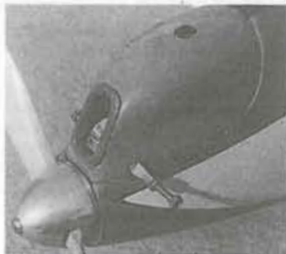
Note the cowl on this 60-inch-span, .60-size biplane. The rubber inlet air restrictor prevents the engine from being over-cooled when flying during winter.
