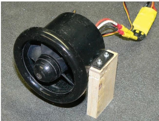
The width of the fuselage is determined by the size of the ducted fan unit you use. Here the motor mount rail and spacer have been screwed to the attachment tab on the EDF unit.
