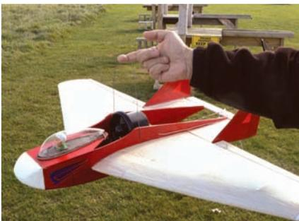
I checked the model's balance with a piece of wire bent like this and inserted into holes in the side of the fuselage. Works great!
