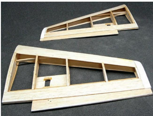
The wing panels are easy to build and easy to assemble. There are building and alignment tabs on the ribs to keep them straight during construction. These are removed before sheeting is installed on the wings.
