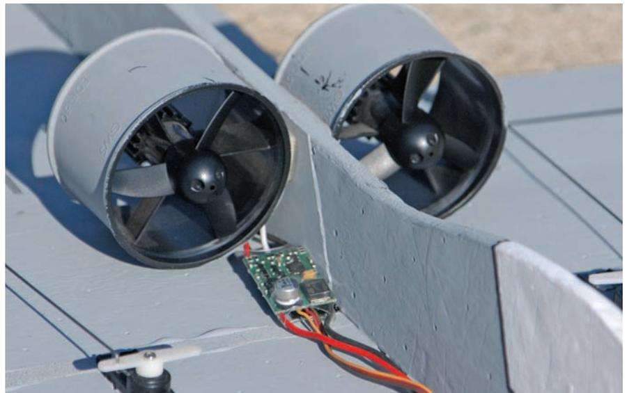
This closeup shows the twin EDF installation. The ducted-fan unit housings are simply glued into place with epoxy onto balsa support blocks that are in turn, epoxied to the plywood doublers on the sides of the fuselage.
