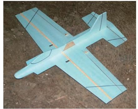
The basic airframe is fully assembled and ready for equipment installation.
