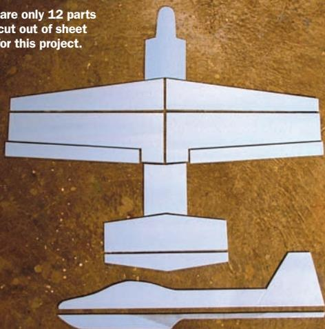
The major subassemblies including the wing, spar, stabilizer and filler pieces—all glued together. The ailerons and elevator have been hinged into place and the upper and lower fuselage pieces are ready to be glued in place.
