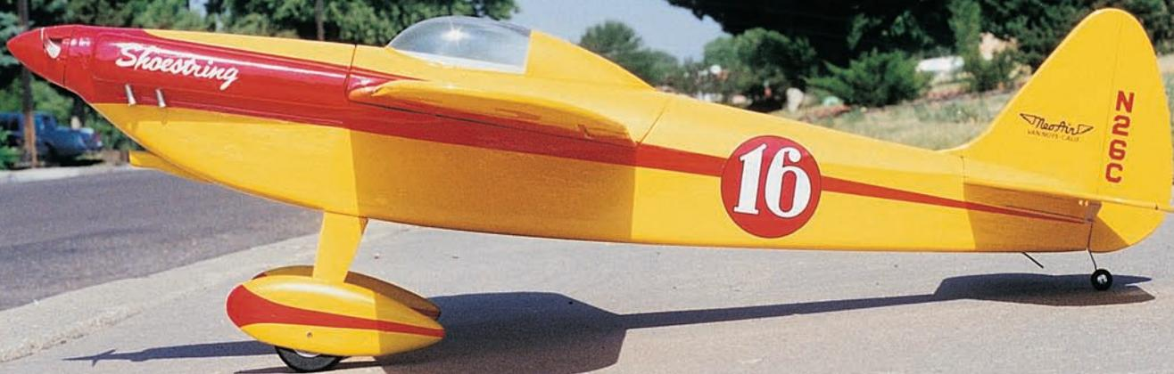
Sig 1/16 x 1 x 10-inch landing gear blank, drill and shape the gear as shown on the plans. Drill and tap the plate for the 8-32 bolts and attach the landing gear. Now cut out, assemble and shape the wheel pants to complete the basic fuselage.
