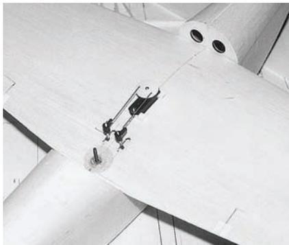
The aileron servo is attached to the center of the Shoestring wing, which is attached to the fuselage with a 3/4-inch-long 4-40 bolt and blind nut.
