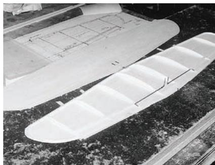
The dihedral is built into the bottom wing skin by using the jigs shown on the plans. The ailerons are controlled via the torque tubes; be sure they fit well before you glue them into place.
