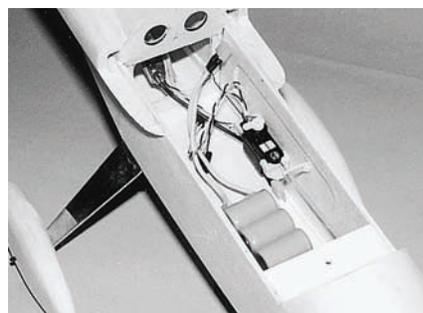
Use the battery as ballast to properly adjust the CG. The battery is held in place with Velcro.
