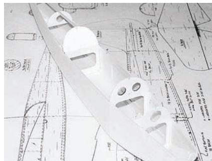
The Shoestring fuselage is fairly easy to assemble. The tail surfaces are sheet balsa. The elevator is hinged with UltraCote after the tail pieces have been covered.
