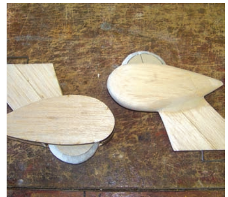
The wheels are assembled into the pants, then the assembly is carved and sanded to final shape.
