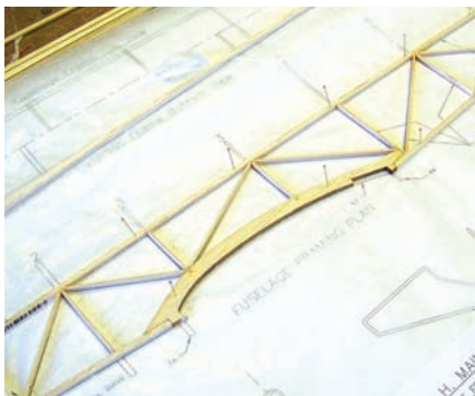
The two fuselage side frames are built directly over the plans.
