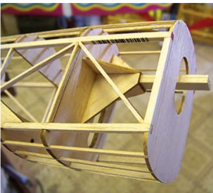
The motor mount assembly is assembled and then glued to the firewall. The right thrust is built into the mount gussets to insure its accuracy.
