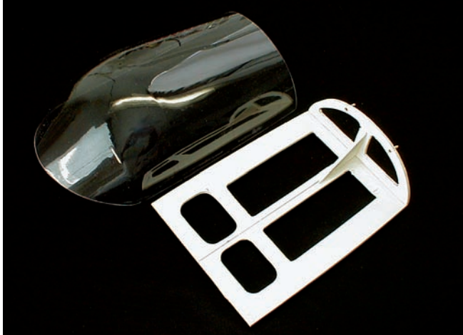
Clear molded cabin section is glued to frame; the entire assembly is easily removable for battery and radio equipment access without having to remove the wing.
