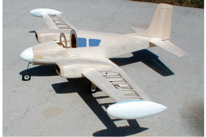
All framed up awaiting final sanding and covering. Cabin section has not yet been removed to accept final configuration clear parts. Note molded cowls, tip tanks and nose cap available from hobbyhangar.com.
