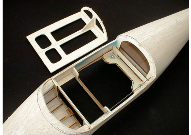
Removable cabin section is retained by short lengths of dowel at the aft end and a single nylon screw at the front edge. 3S 2100mAh LiPo battery will be located as far forward as possible.
